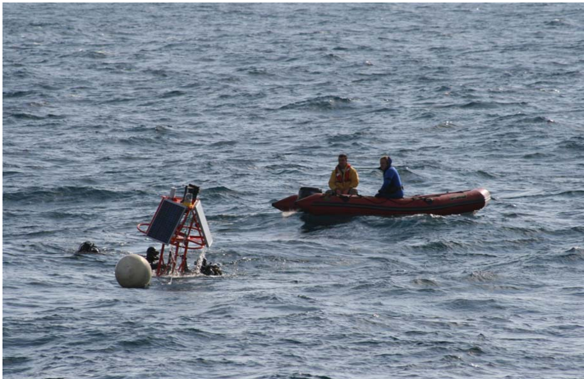
Figure 1. Top of the buoy, partly underwater because of strong currents, inspected from divers.
